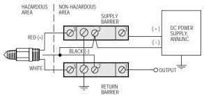
Supply and Return Zener Barriers used with GEMS ELS-1100 Series electro-optical level switch.
