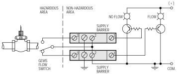
Used with GEMS flow switch located in a hazardous area for flow/no flow indication.
